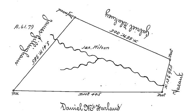
The above is the traight of a Survey Situate in Greene Country on the Waters of the South fork of Sen Hole Creek, containing 364 acres and 96 perches with allow of Dix processor troads to the which was made on the 18th of Hoarch 1797 in pursuance of a Warrant Granted to James Wilson for 373 acres on the 12th of Jam's 1797
